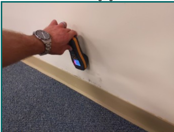
Wet conditions and suspected mold staining at middle building rear room
