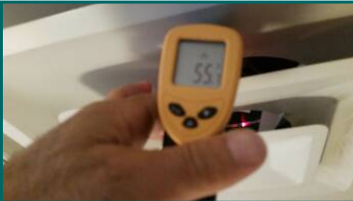
AC has acceptable temperature drop at 2nd floor left side unit
